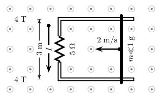
Calculate the applied force required to move the bar to the left at a constant speed of 2 m/s. Answer in units of N.
