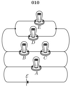
Rank the brightness of the identical bulbs in the following circuit. Hint: You may find it helpful to work out the currents through the bulbs for the case V=1 V, and R=1  $\Omega$  for all the bulbs, then compare the currents.
