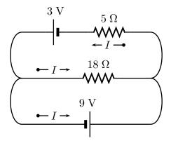
Find the current through the 5  $\Omega$  resistor and the 3 V battery at the top of the circuit. Answer in units of A.
