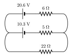
Find the current through the 22  $\Omega$  lower-right resistor. Answer in units of A.
