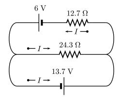
Find the current through the  $12.7 \Omega$  resistor and the 6 V battery at the top of the circuit. Answer in units of A.
