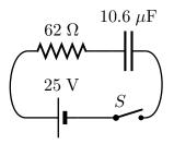
How long after the switch is closed does the voltage across the resistor drop to  $V_f = 16 \text{ V}$ ? Answer in units of s.
