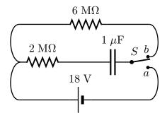
Find the voltage across the 2 M $\Omega$  center-left resistor at time  $t_1=3$  s. Answer in units of V.
