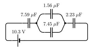
Find the equivalent capacitance of the circuit. Answer in units of  $\mu$ F.
